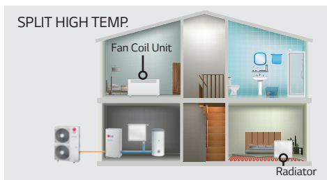
Image above: Example diagram showing different heat emitters, for illustration only.
